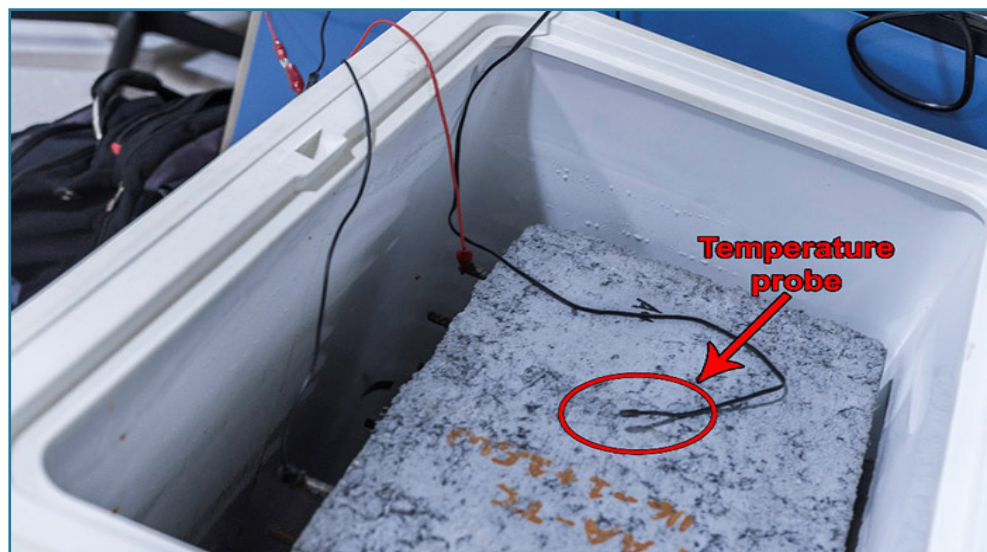
A concrete test slab is seen here in a deep freezer at the University of Nebraska-Lincoln.
