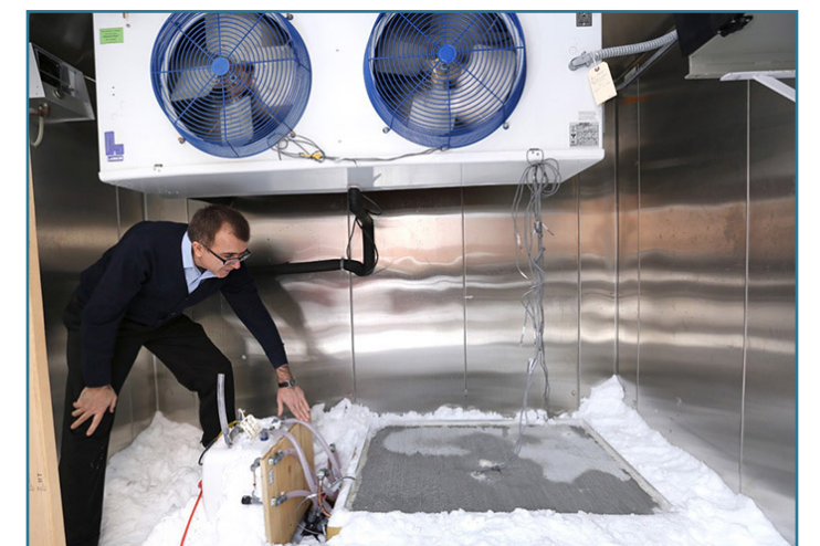
Iowa State's Halil Ceylan checks a test slab that uses heated pavement technology to melt snow and ice. One of the goals of the research project is to help smaller airports clear runways during winter storms. Photo by Christopher Gannon.
