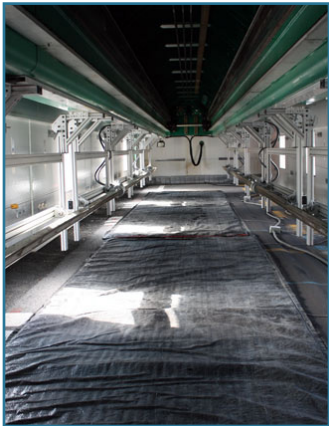
Heating panels run along each side of the path that the wheel follows in the HVS-A. (Photo: ATO)
